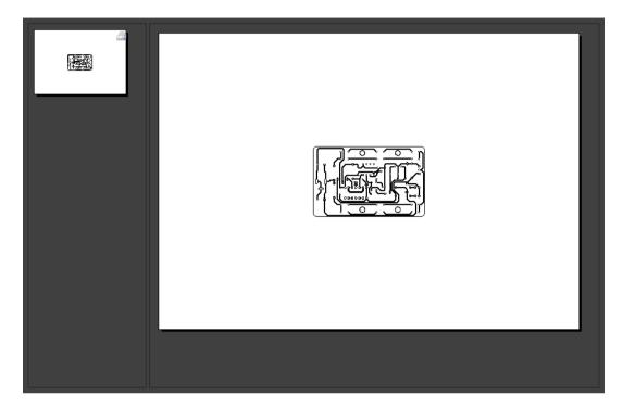
12) If you want to create a double layer design you should repeat step 9 but instead off removing the top layer you need to remove the bottom layer. Keep in mind you need two different stencils for top and for bottom layer.
