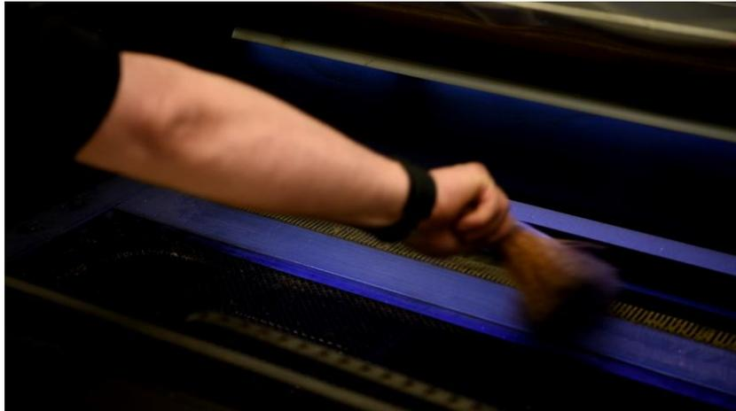
The smoke gets extracted through the raster in the back of the machine.
